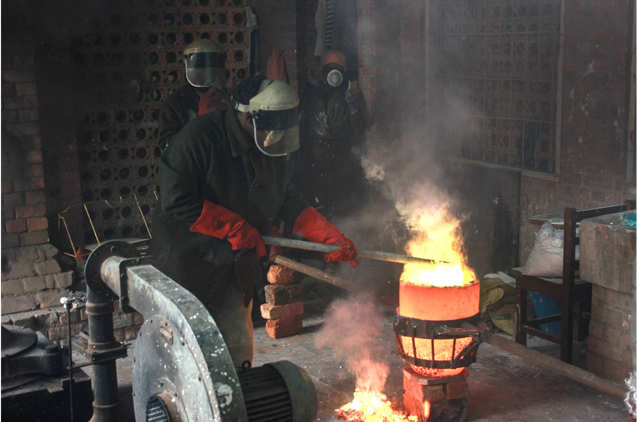
Metal casting process where molten metal is poured into molds illustrating the technique shared by African metalworkers that enabled production of complex brass and bronze items (e.g., tools, ornaments) through lost-wax casting techniques. Photo credit: Samson iron via Wikimedia Commons.
